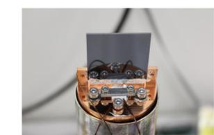
Si(111) substrate (40 × 40 × 1 mm) connected to a 4 K He refrigerator. Indium solder is used to cool the Si substrate down to 6 K.
